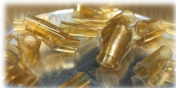
Figure 3: PET sample with discolouring by remaining adhesive
