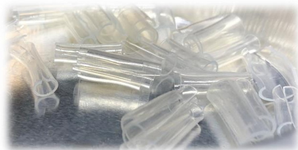
Figure 2: PET sample without discolouring after roasting (test passed)
