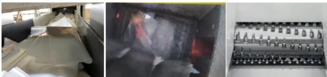
Fig. 25: S GRAN 95 impressions (left: material feed; middle: shredding unit; right: screw)
