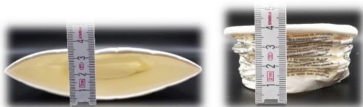
**Figure 2:** Evaluation of the compressed height after the test (examples)
